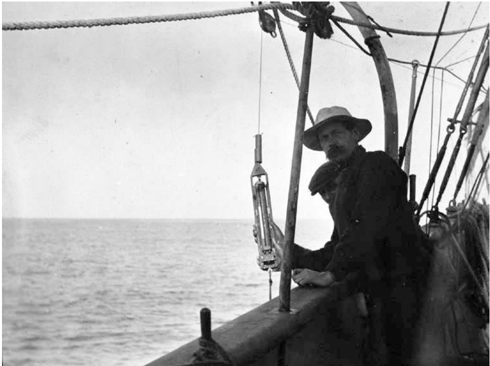
Water sampling onboard F.I.S. Endeavour . Photo in the J. K. Davis Collection, State Library of Victoria
